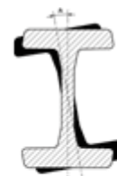
bow on length (twist) A max = 0.5°/meter
