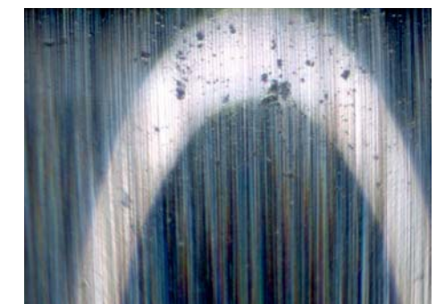
Indentations in raceway caused by particles
